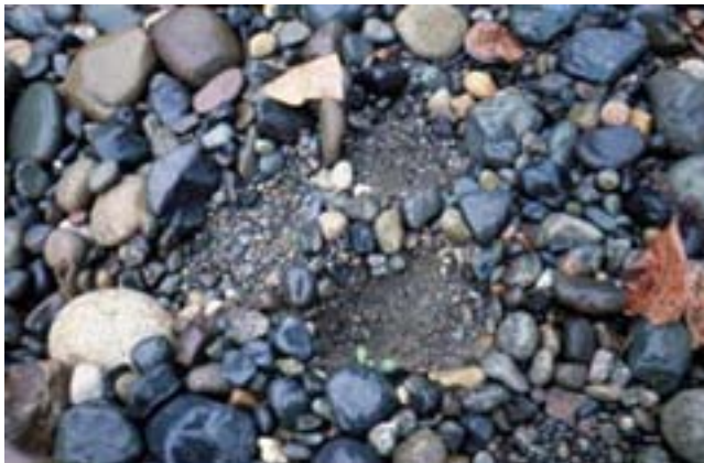
Figure 7-8 Subsurface layer exposed after removal of three cobbles from the armour layer
