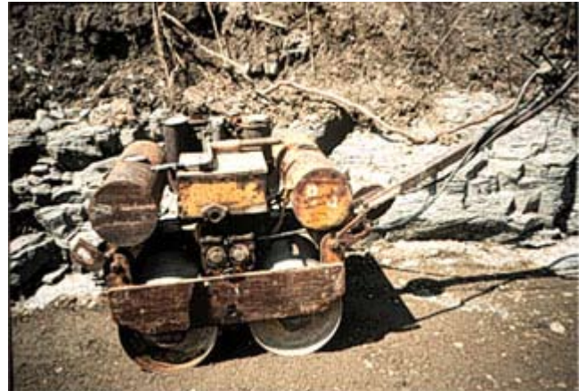
Figure CS4-7 Manually directed vibrating drum roller
