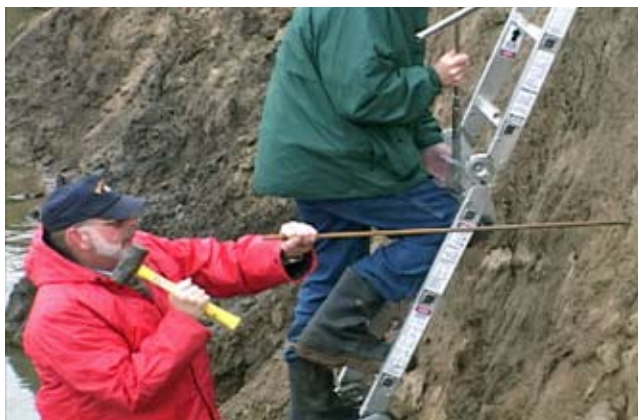
Figure CS9-17 Installing bank erosion pins
