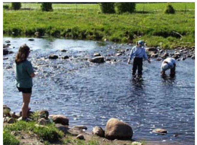
Figure CS3-8 Performing the Wolman pebble count
